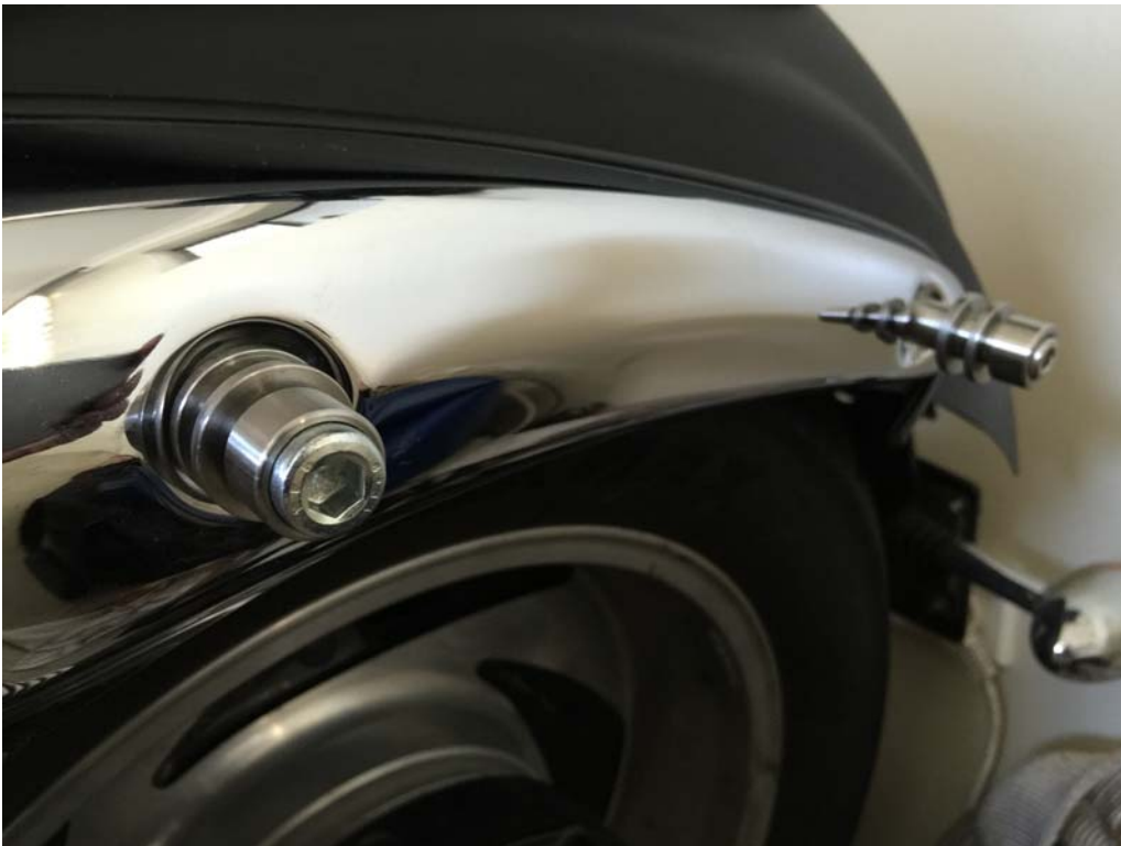
Replace Standard Bolts with the kit provided. The M10 Cap Screw Bolt kit replaces the front bolt The M8 Cap Screw Bolt kit replaces the rear bolt This is how it looks when the rack is NOT fitted.
